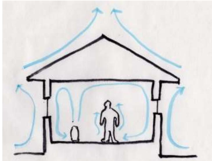
Heat transfer between solid and fluid (air)
